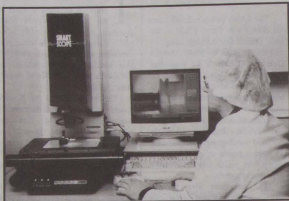
An inspector in KippGroup's clean room uses the "Smart Scope," an advanced video inspection device which magnifies parts up to 200 percent to ensure consistent quality.
