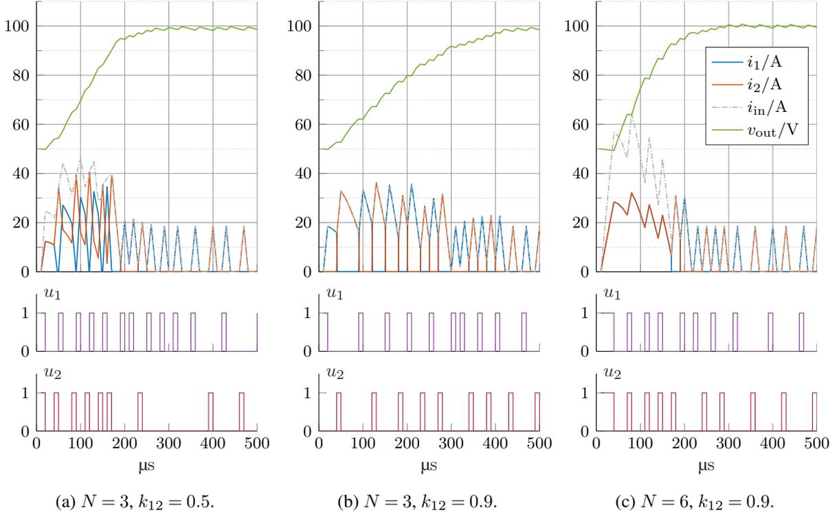
Fig. 14: Start-up behavior of the interleaved dc-dc boost converter for different  $N$  and  $k_{12}$ .
