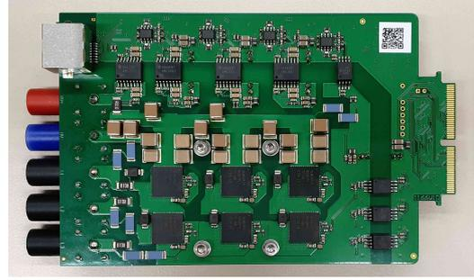
Fig. 11: GaN adapter card bottom side.
