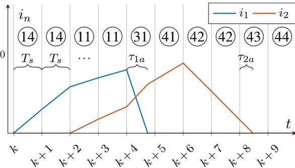
Fig. 4: Illustrative subset of modes of interleaved boost converter.
