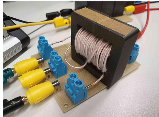
Fig. 9: Coupled inductors prototype.
