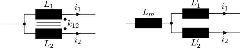
Fig. 2: Coupled inductors and equivalent Y-model.
