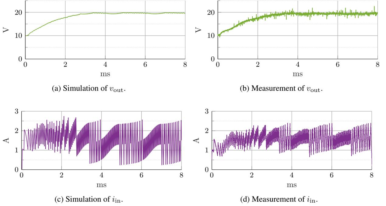
Fig. 12: Comparison between simulation and experimental measurements.
