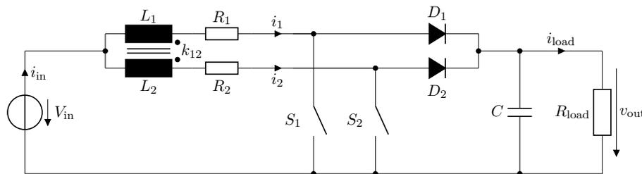
Fig. 1: Interleaved dc-dc boost converter with coupled inductors.
