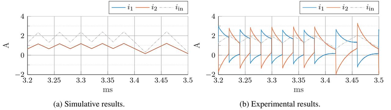
Fig. 13: Branch currents  $i_1$  —,  $i_2$  — and input current  $i_{in}$  - - -.
