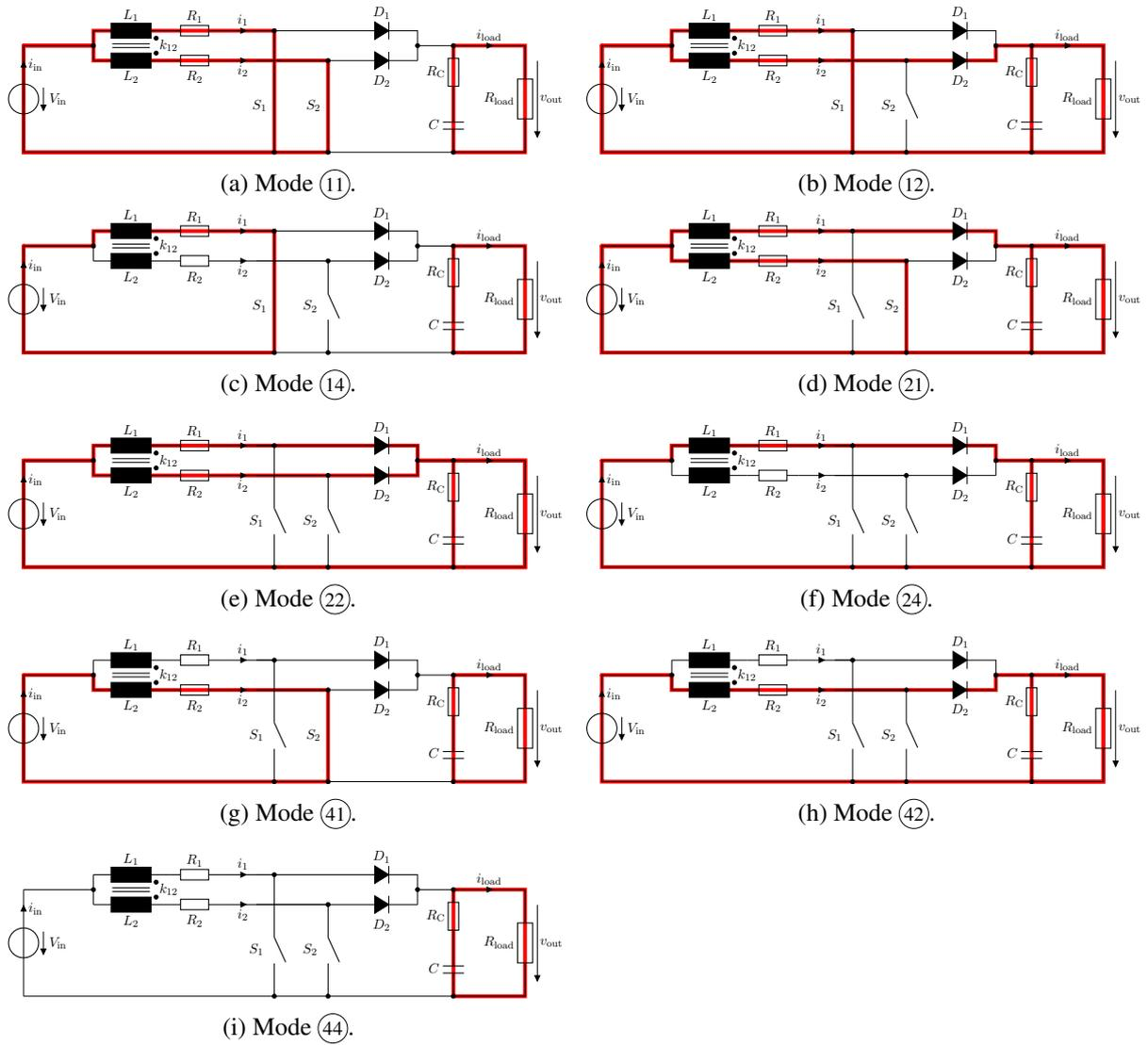
Fig. 5: Active current paths (—) of the interleaved boost converter in different operating modes.
