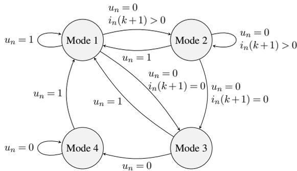
Fig. 3: State machine of branch  $n$  [7].
