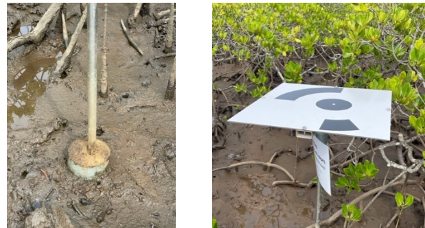
Figure 5. Photographs of the first target placed in our study area for photogrammetric acquisitions (left : concrete base; right : target on the top of the steel).
