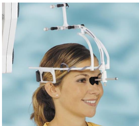
Abbildung 7: Messsystem Zebris ultrasound-based motion analysis system (Zebris Medical GmbH, n.d)
