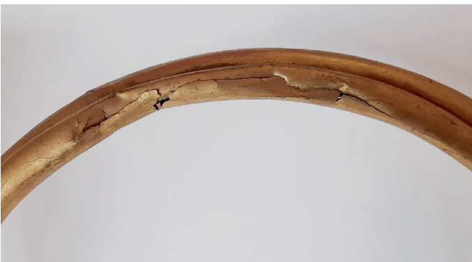
FIGURE 2 Crumpled tubing due to impact on weakened brass (photo courtesy of Richard Seraphinoff)
