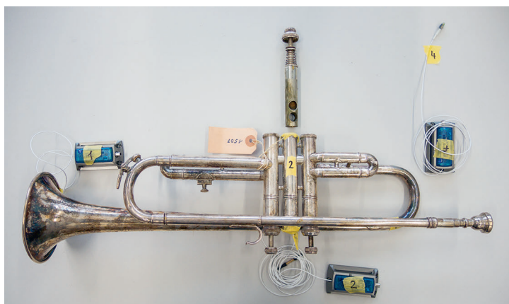
FIGURE 2 Test arrangement using data loggers for climate testing on a trumpet
