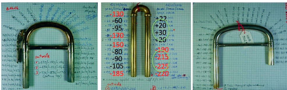
FIGURE 5 Results of corrosion potential measurements performed with the sensor inside the tuning slides. The numbers here indicate the potential measured at a given position after 30 seconds, 1 and 2 minutes. Measurements were taken at a distance of 1 cm in the left and right arm of the tuning slide. Potential of the sensor vs Ag/AgCl sat = -170 \pm 10 mV. a) HKВ 5004.2 – b) HKВ 5009.2 – c) HKВ 5025.1
