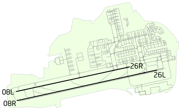
Figure 3. Apron and terminal layout of London–Gatwick Airport.
