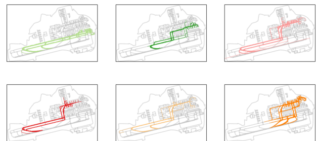
Figure 12. Cluster subset based on three features (latitude, longitude and ground speed) and 50 samples per trajectory. The top right (pink) and bottom left (red) correspond to similar spatial flows but different ground speed profiles (see Fig. 13).
