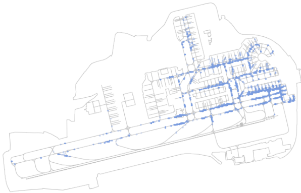
Figure 11. Density map of positions of aircraft with zero ground speed.
