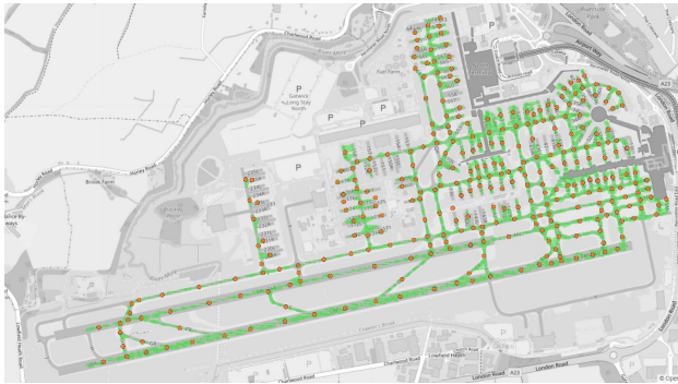
Figure 5. Density-based clustering of transmitted aircraft positions to derive airport infrastructure, such as parking positions or operational network (e.g. taxi way connections) validated against information from OpenStreetMap.
