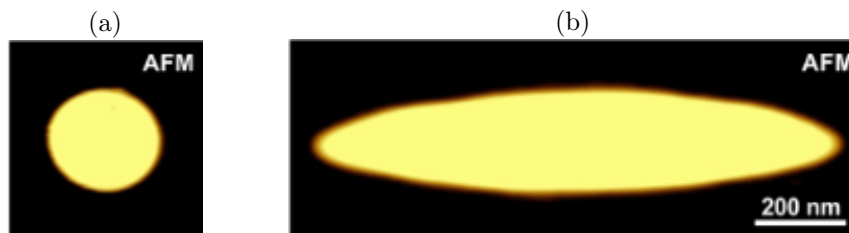
Figure 7.1: AFM micrograph of the initial and elongated colloid in the presence of linearly polarized light. The light-induced elongation ratios is about 5. Modified and reproduced from Ref. [52].
