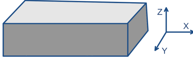
Figure 6.4: The top surface represented with the light gray colour is free to move in all three directions and the all four side surfaces represented with dark grey color are restricted to move in the normal direction.
