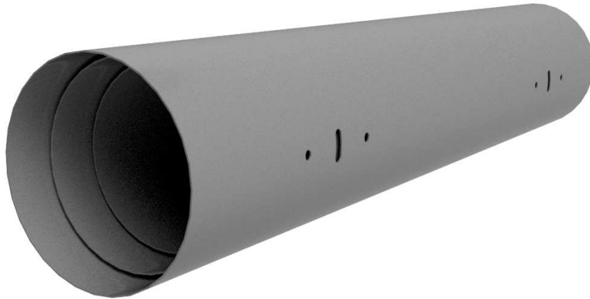
Figure 2.5: Magnetic shield used to mitigate Earth’s magnetic field. The outermost length is 485 mm, the innermost is 400 mm. The inner cylinder diameter is 8 cm with a 5 mm gap between layers. Thru holes were made to allow electronic connections to the RF loops.
