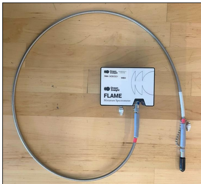
Figure 4.4: Spectrometer used to measure emission spectra.
