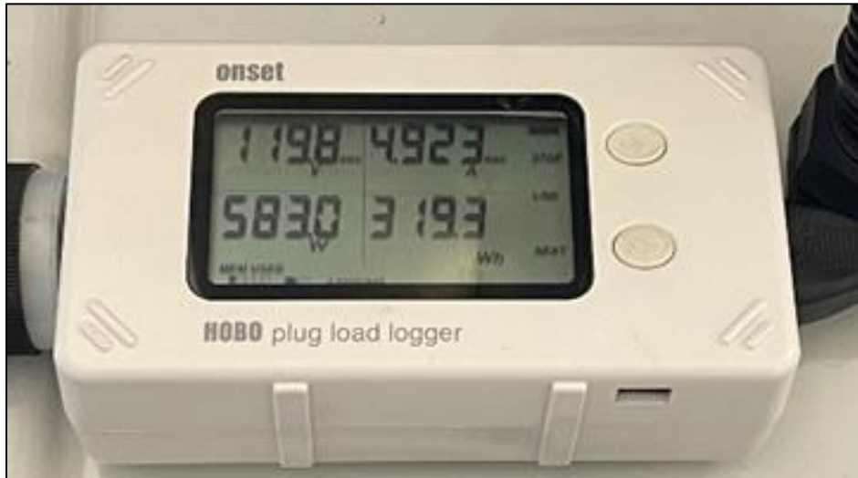
Figure 4.24: HOB0 plug load monitor and logger that displays real time power consumption of the device
