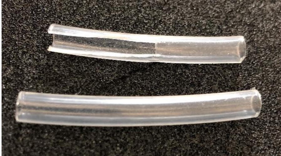
Figure 4.11: The top tube sample is trimmed for insertion into the single-wall insertion port. The bottom tube sample is untrimmed for double-wall transmittance testing.
