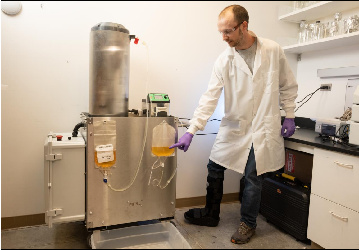
Figure 5.8: Bulk zika virus solution flowing from the inlet bag (see bag being pointed to), through the VacciRAPTOR illumination chamber, and out into to the outlet bag. Credit: John Eisele/Colorado State University Photography
