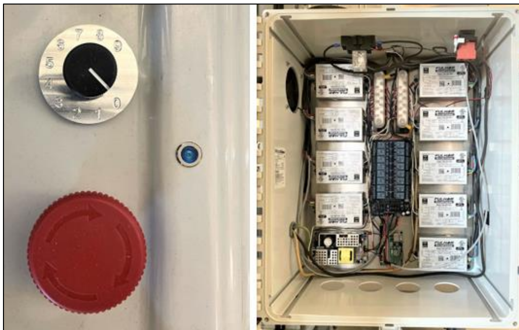
Figure 4.23: Emergency stop button (red knob), lamp program selector (black knob), and layout of lamp ballasts and other electronic equipment within the VacciRAPTOR.
