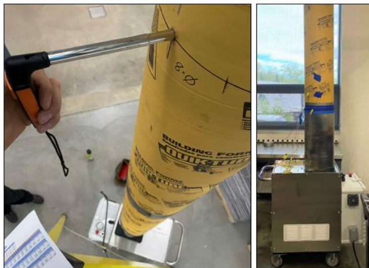
Figure 4.20: Volumetric airflow test setup. The inside diameter of the large yellow tube is equal to the diameter of the VacciRAPTOR's airflow field (inside diameter = 26cm, length = 10x inside diameter, flow measurement location = 8x inside diameter downstream).
