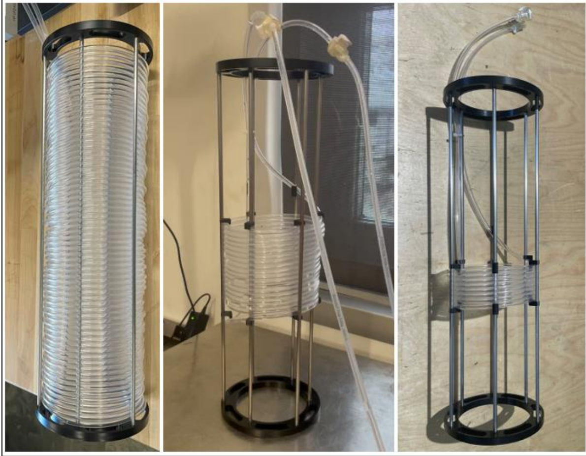
Figure 4.13: Images of the scalable reactor coil design (left = full size, middle = quarter size, right = eighth size). Treatment capacity of the VacciRAPTOR scales directly with the size of the tubing coil. Larger coils allow for greater treatment capacities than smaller coils.
