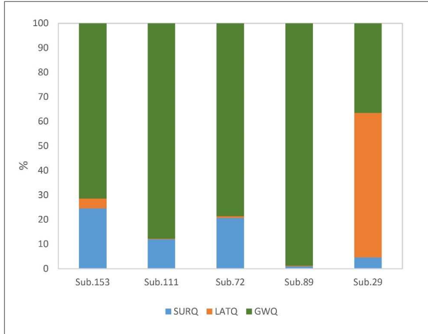
Figure 2.8. Percentage of surface runoff (SURQ), lateral flow (LATQ) and groundwater return flow (GWQ) contribution to water yield in subbasins 153, 111, 72, 89 and 29.
