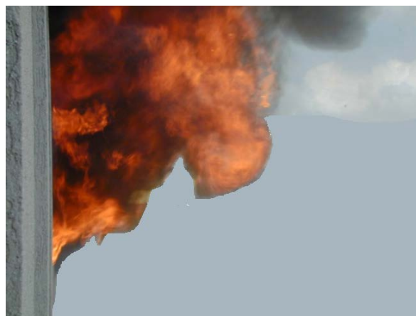
Figure 8. Ejected façade fire from compartment window due to the ventilation
