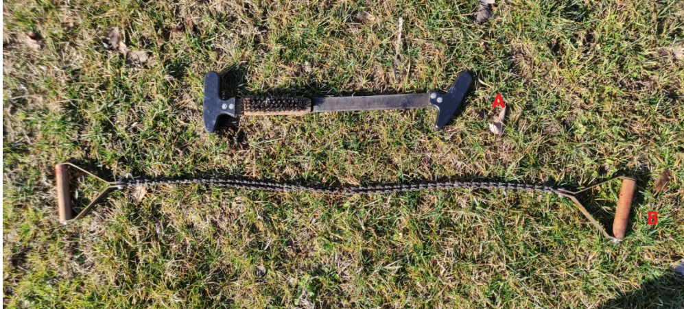
Figure 3 - Manual tools used for girdling: Cutting girdler (A) and Chainsaw girdler (B).
