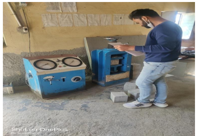
Fig. 4 Performing the compressive test on cubes in compression testing machine
