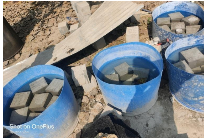
Fig. 3 Curing of concrete
