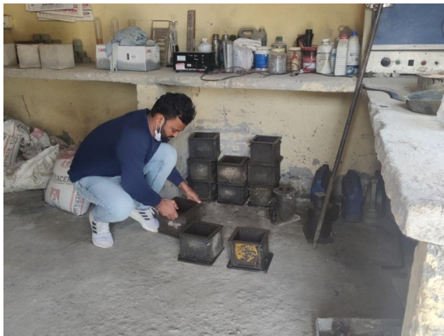
Fig. 2 Casting of cubes
