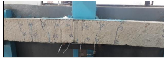
Fig.3 Cracks Pattern of the Beam
