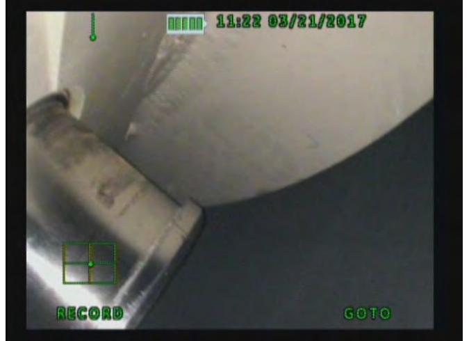
9. Overpack and lifting trunnion
