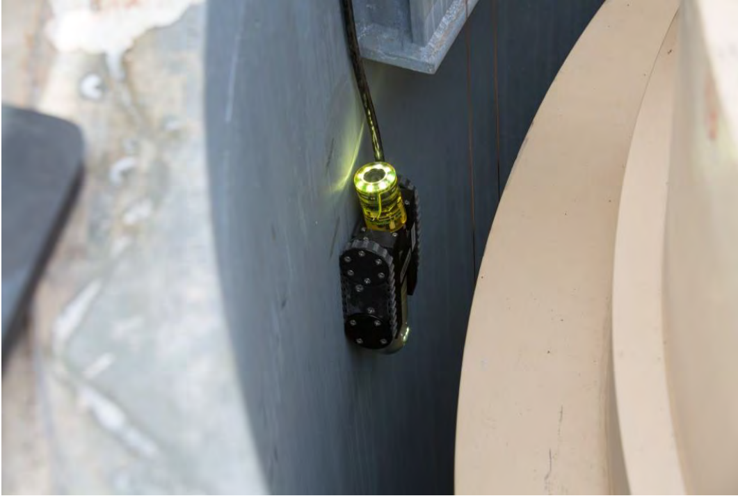
3. Crawler on liner examining overpack
