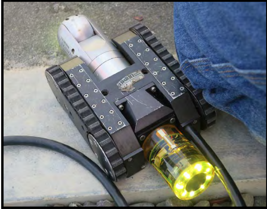
Figure 4: Nanomag™ Magnetic Crawler System
