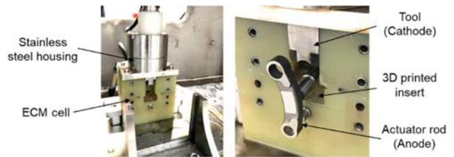
Fig. 4 – ECM setup for insert trial test.
