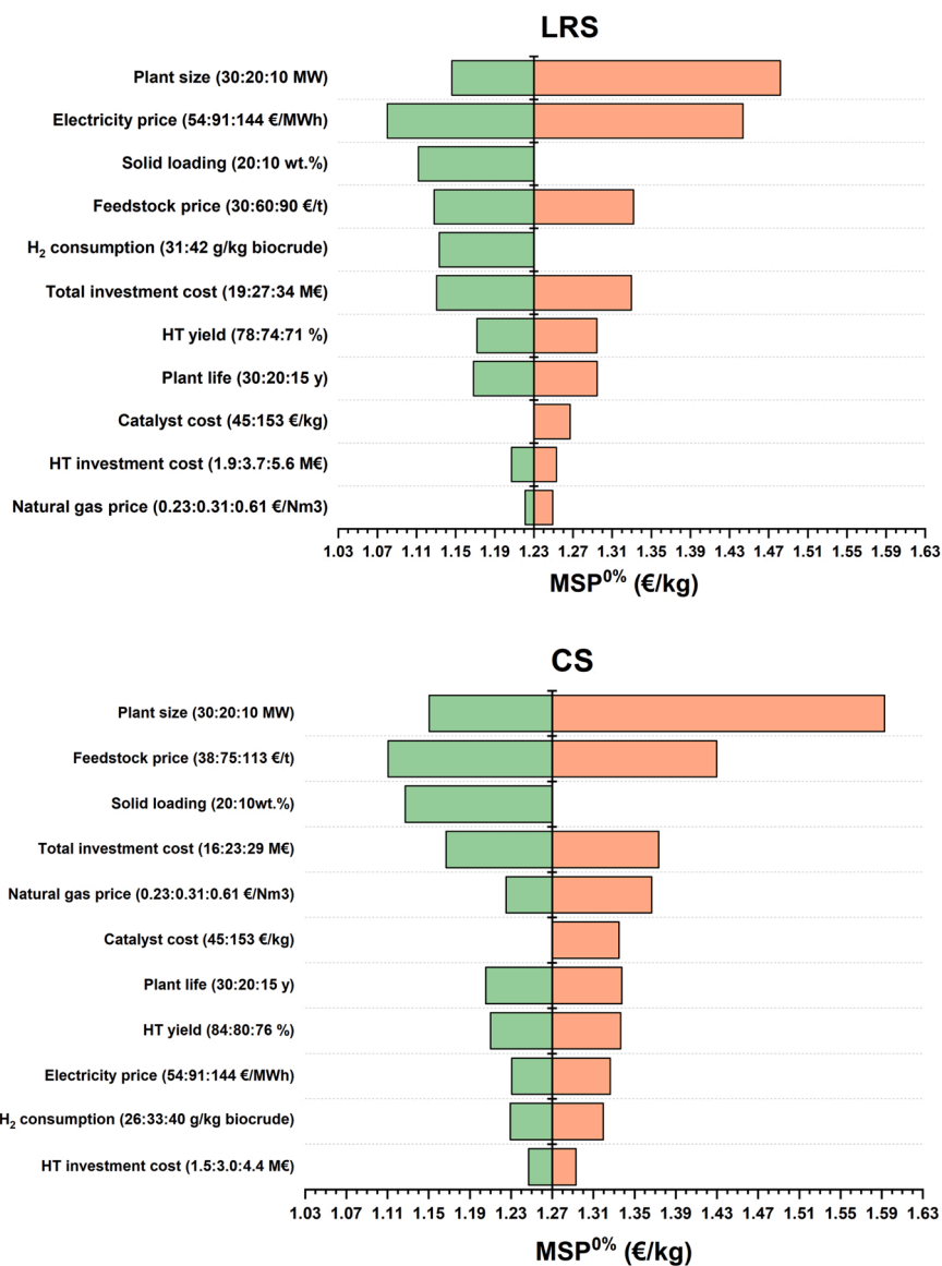
Fig. 6. MSP 0% changes as consequence of the sensitivity analysis performed for the lignin-rich stream (above) and corn stover (below) scenario.
