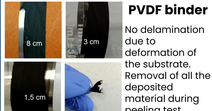
No delamination due to deformation of
