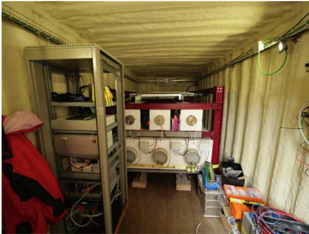
Fig. 2. MazORCA interior. The control and communications electronics cabinet is in the front, and the structure with ORCA’s detectors is in the back.
