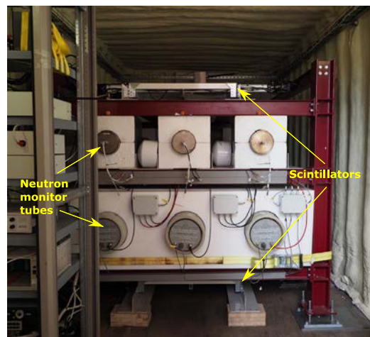
Fig. 2. ORCA setup, including the two MITO devices at the top and bottom and NEMO in between.
