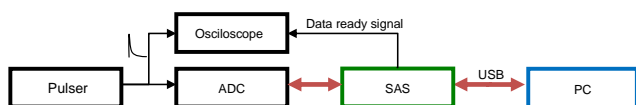
Figure 6. Block diagram used to verify the ADC conversion time. PC is only used to launch and stop SAS software.
