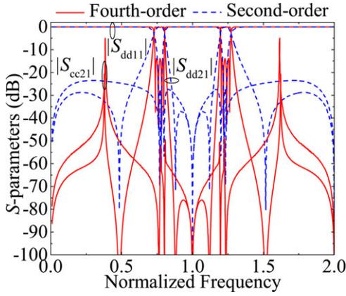
**Fig. 7.** Theoretical differential-mode power transmission ( $|S_{dd21}|$ ), reflection ( $|S_{dd11}|$ ), and common-mode suppression ( $|S_{cc21}|$ ) responses of the proposed fourth-order balanced dual-band BPF in Fig. 6 with  $Z_c = 42\Omega$ ,  $Z_{c1} = 50\Omega$ ,  $Z_{oe1} = 77.5\Omega$ ,  $Z_{oo1} = 31.8\Omega$ ,  $Z_{oe2} = 98.7\Omega$ ,  $Z_{oo2} = 32.5\Omega$ , and  $Z_L = 16.7\Omega$ .
