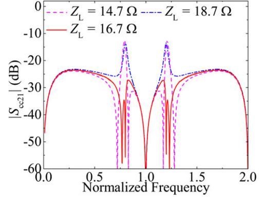
**Fig. 4.** Theoretical common-mode suppression ( $|S_{cc21}|$ ) responses of the corresponding sub-circuit in Fig. 1(c) associated to the proposed second-order balanced dual-band BPF versus different values of  $Z_L$  when  $Z_C = 42\Omega$ ,  $Z_{oe1} = 77.5\Omega$ ,  $Z_{oo1} = 31.8\Omega$ ,  $Z_{oe2} = 98.7\Omega$ , and  $Z_{oo2} = 32.5\Omega$ .
