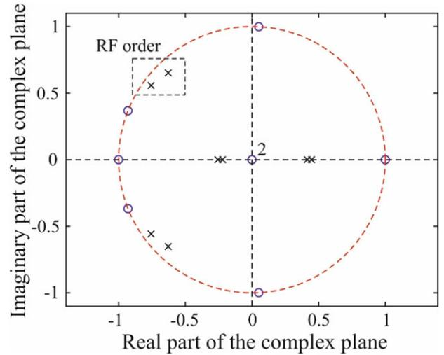
**Fig. 8.** Zero-pole diagram of the digital system associated to the differential-mode transmission scattering parameter of the one-stage balanced dual-band BPF in Fig. 7 (poles are represented with black symbol "x"; zeros are represented with blue symbol "o"; numbers indicate the multiplicity of the root).
