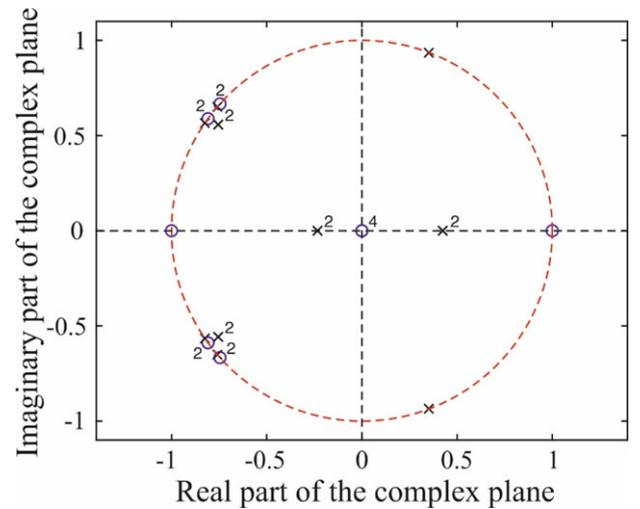
**Fig. 11.** Zero-pole diagram of the digital system associated to the common-mode transmission scattering parameter of the two-stage balanced dual-band BPF in Fig. 7 (poles are represented with black symbol “x”; zeros are represented with blue symbol “o”; numbers indicate the multiplicity of the root).
