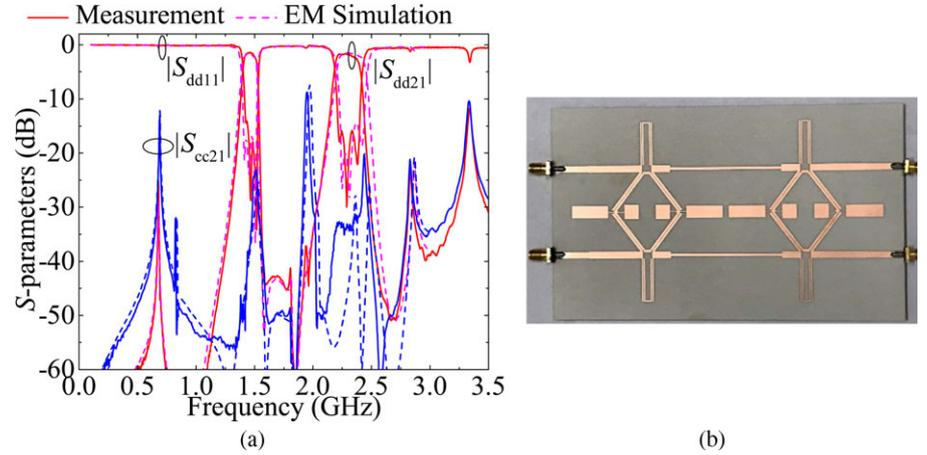
**Fig. 13.** Manufactured fourth-order balanced dual-band BPF prototype with its layout in Fig. 11. (a) Simulated and measured differential-mode power transmission ( $|S_{dd21}|$ ), reflection ( $|S_{dd11}|$ ), and common-mode suppression ( $|S_{cc21}|$ ) responses. (b) Photograph.
