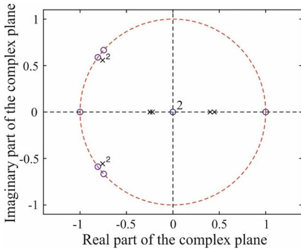
**Fig. 9.** Zero-pole diagram of the digital system associated to the common-mode transmission scattering parameter of the one-stage balanced dual-band TFS in Fig. 7 (poles are represented with black symbol “x”; zeros are represented with blue symbol “o”; numbers indicate the multiplicity of the root).
