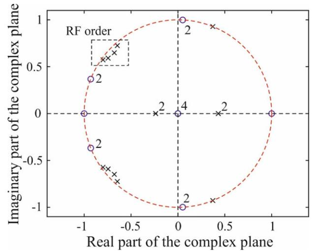
**Fig. 10.** Zero-pole diagram of the digital system associated to the differential-mode transmission scattering parameter of the two-stage balanced dual-band BPF in Fig. 7 (poles are represented with black symbol “x”; zeros are represented with blue symbol “o”; numbers indicate the multiplicity of the root).
