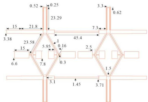
**Fig. 12.** Layout of the implemented fourth-order balanced dual-band BPF based on its relevant four-port equivalent circuit in Fig. 6 (all the indicated physical dimensions are given in mm).
