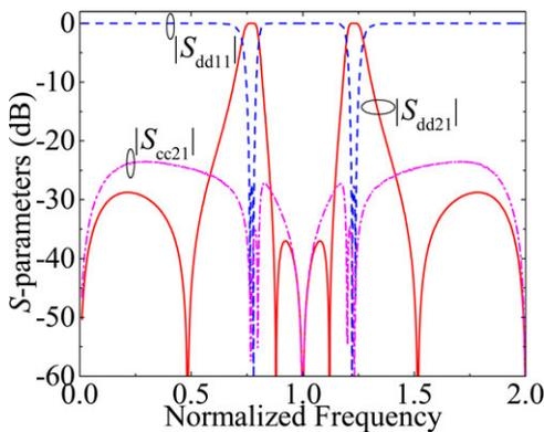
**Fig. 2.** Theoretical differential-mode power transmission ( $|S_{dd21}|$ ), reflection ( $|S_{dd11}|$ ), and common-mode suppression ( $|S_{cc21}|$ ) responses of the proposed second-order balanced dual-band BPF in Fig. 1(a) with  $Z_C = 42\Omega$ ,  $Z_{0e1} = 77.5\Omega$ ,  $Z_{0o1} = 31.8\Omega$ ,  $Z_{0e2} = 98.7\Omega$ ,  $Z_{0o2} = 32.5\Omega$ ,  $Z_L = 16.7\Omega$ , and  $\theta(f_0) = \theta_1(f_0) = \theta_2(f_0) = 90^\circ$  (reference impedance  $Z_0 = 50\Omega$ ).
