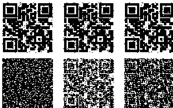
Figure 10. Extracted watermarks under Gaussian attacks. The first row corresponds to KS1Ms, KS2Ms, and KS3Ms while the second row corresponds to KMs, FrCMs, and FrCMMs.
