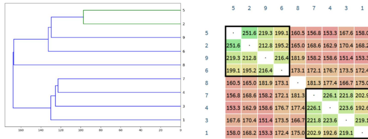
Figure 4.11: Dendrogram (left) and global similarity matrix (right) for SensoGraph with distances. The matrix is rearranged according to the result of the dendrogram, so that the groups obtained appear as submatrices with similar colors (framed).
