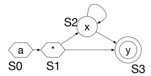
Figure 5.1: Illustrating an NFA that accepts a\*.x\*y.  $S_0$  and  $S_1$  are *all-input* starting states, which are always active in the execution.
