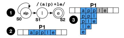
Figure 5.6: Synchronous execution identifies disjoint patterns; Patterns identified by different threads in asynchronous execution may overlap.
