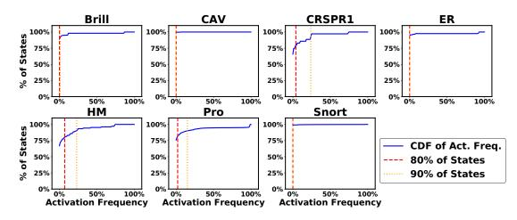
Figure 4.6: The activity profile of the states. For the majority of applications, 80% of non-starting states are activated for only less than 1% of the processed symbols.
