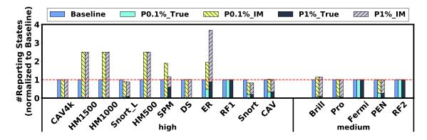
**Figure 3.12**: Comparison of number of reporting states: "IM" stands for intermediate reporting states. "True" stands for original reporting states on BaseAP mode. "P" stands for profiling. (c) 2018 IEEE.
