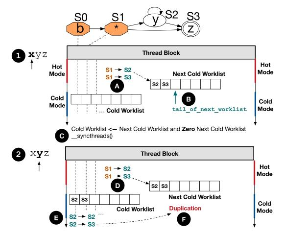
(a) An illustrative example for our activity-based processing scheme: orange shaded states are hot (active) states mapped to threads and cold (inactive) states are handled via worklist. The *active bitset* for hot states is not shown.
