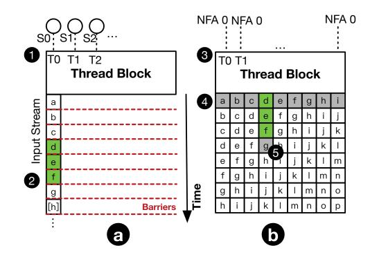
**Figure 5.2**: Revisiting traditional synchronous automata processing on GPU (a) and the basic idea of ASYNCAP (b). The executions try to find pattern **def** in an input stream **abcdefg...**
