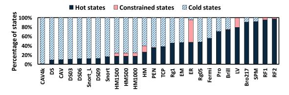
**Figure 3.8**: Constrained states are cold states but configured on the AP due to the constraints in our topological-order-based partitioning scheme. Consequently, some AP resources are underutilized with a few applications. © 2018 IEEE.
