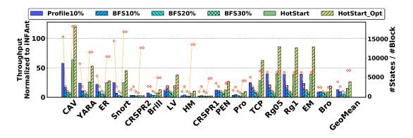
Figure 4.8: Throughput sensitivity to the selection of hot states. Detailed evaluation methodology is in Section 4.6. HOTSTART (or HOTSTART\_OPT, an optimized version) has the best performance among these selection schemes. Hence, we choose the always-active start states as hot states.
