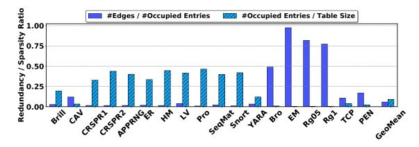
Figure 4.3: Two metrics showing the redundancy (#edges/#occupied-entries) and sparsity (#occupied-entries/table-size) in the transition table. Lower is worse.
