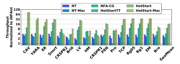
Figure 4.13: Performance sensitivity to Volta GPU Architecture. Both HOTSTART-MAC and HOTSTART show more than  $15 \times$  speedup over INFANT, indicating their effectiveness on newer GPU architectures.
