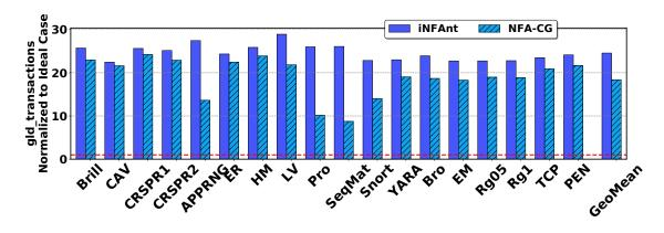
Figure 4.2: The data movement normalized to the ideal cases: two prior schemes use  $25 \times$  and  $18 \times$  compared to the ideal case where only the input stream is loaded. The evaluation methodology is discussed in Section 4.6.
