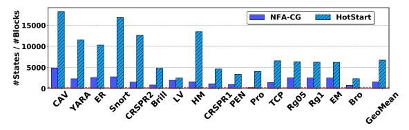
Figure 4.12: Effect on the number of NFA states per thread block (a proxy for compute utilization). More states are handled per thread block in HOTSTART.
