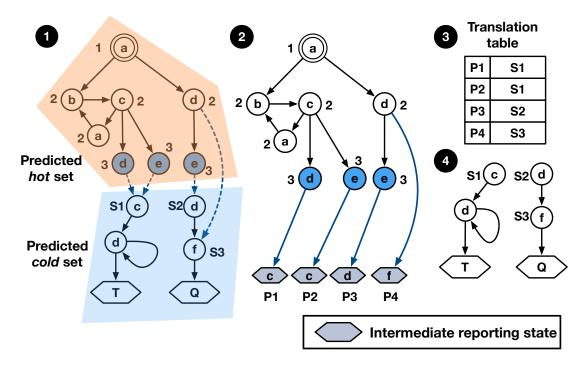
Figure 3.7: Partitioning an NFA by the partition layer. © 2018 IEEE.
