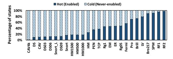
**Figure 3.1**: A large portion of NFA states are cold (never-enabled) but are still configured on the AP leading to its underutilization. (c) 2018 IEEE.
