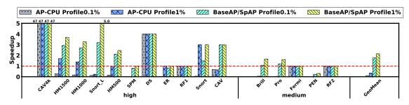
(a) Speedup with AP–CPU and BaseAP/SpAP execution using 0.1% and 1% profiling input (capacity = 24K).
