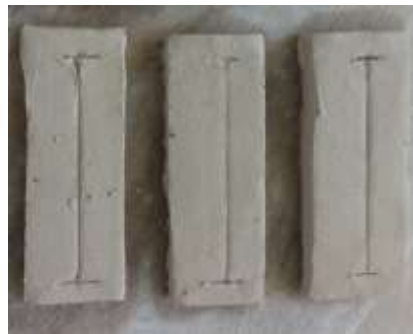
Fig. 2: The process of shrinkage test using a test bar bar slab porcelain clay
