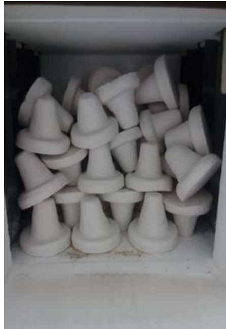
Fig. 3: Bisque body was fired in MV Muffle Furnace 1400
