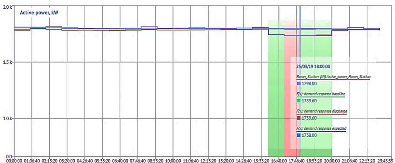
Fig.5. Modeling the load reduction on the MFU of a mining enterprise for the day ahead
