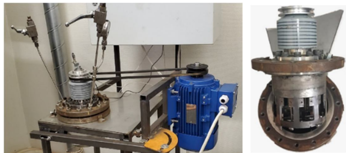
Fig.5. Autoclave for dynamic corrosion testing
