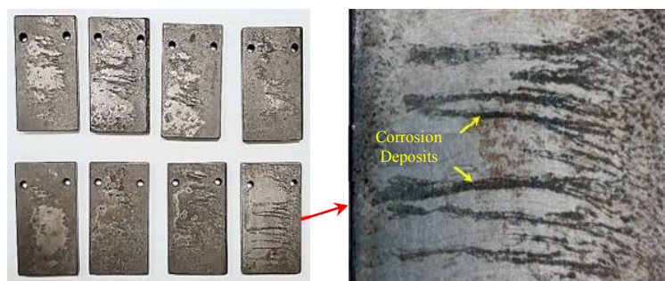
Fig.6. Samples after autoclave testing
