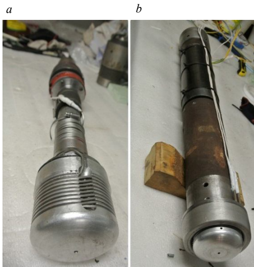
Fig.3. Model of thermohydraulic reamer-drilling tool: TRDT II (a); TRDT I (b)
