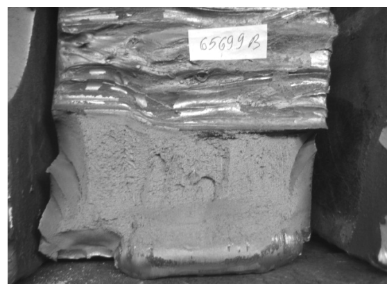
Fig. 3. Cross-sectional view of technological samples from the top and bottom of a sheet 100 mm thick, made of a sheet ingot of high-strength hull steel weighing 20.4 tons.
