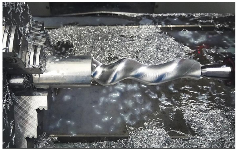
Fig.8. Screw surface machined according to the proposed strategy
