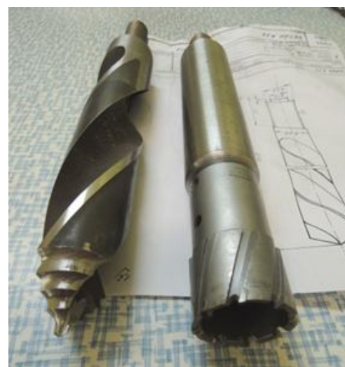
Fig.8. Graduated drill and drilling bit [6]
