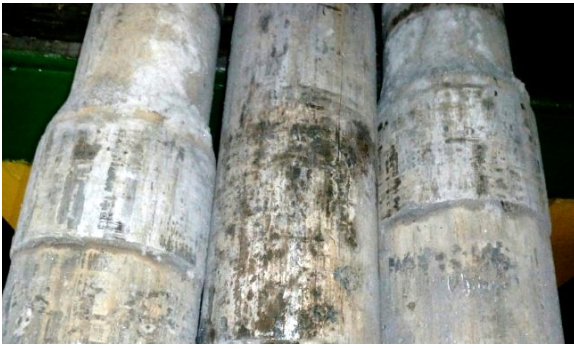
Fig.6. Fragments of the SDP locks without surfacing (in the middle) and with hardbanding
