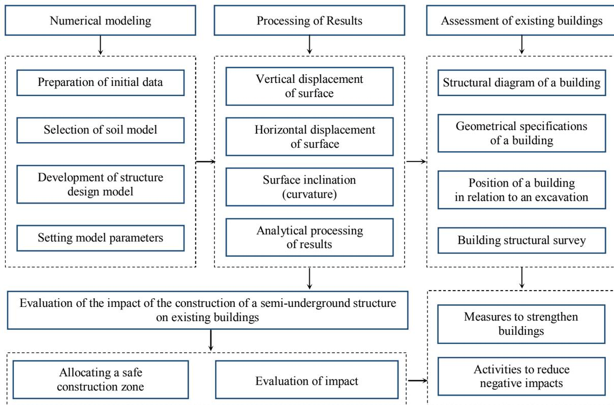
Fig. 1. Algorithm for calculating semi-underground structures
