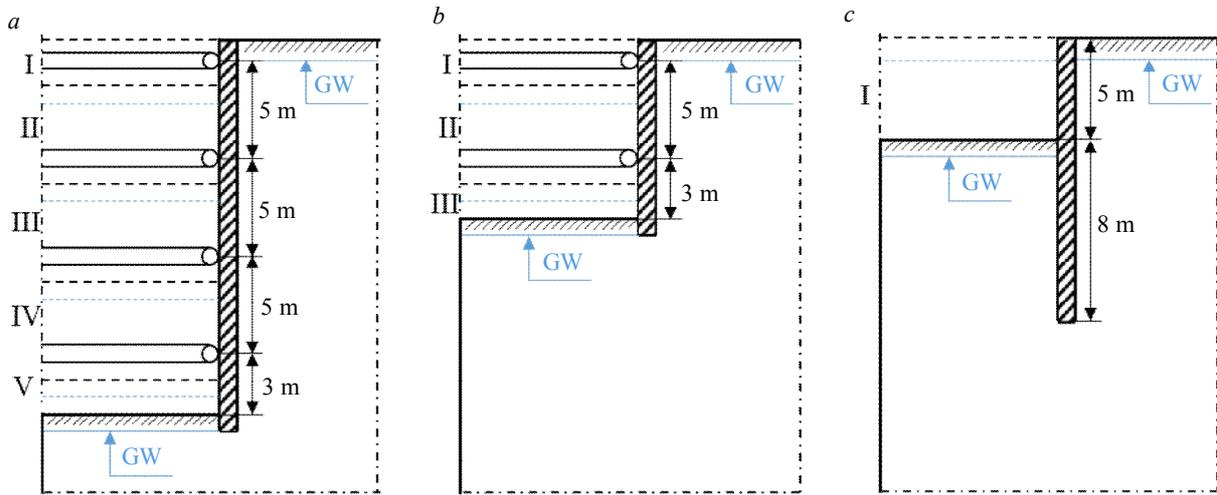
Fig.3. Excavation models: a-c – the depth of an excavation is 19, 9 and 5 m respectively; the cantilever pattern I-V – excavation stages
