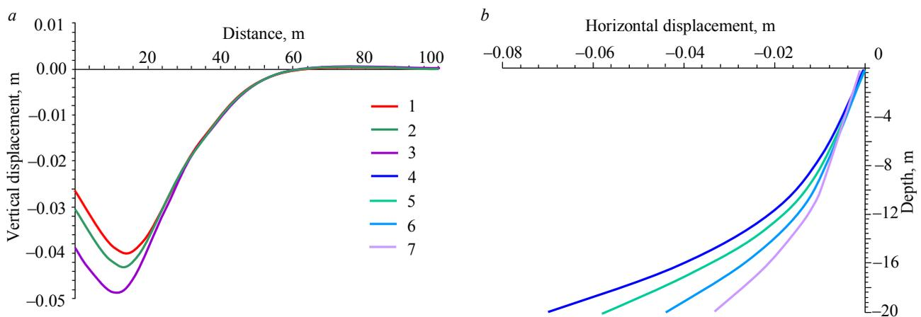
Fig.4. Graphs of vertical (a) displacements of surface in clay N 1 with different depths of «slurry trench» (model 1) and diagrams of horizontal displacement of «slurry trench» (b) with different clays (models 1-4)
