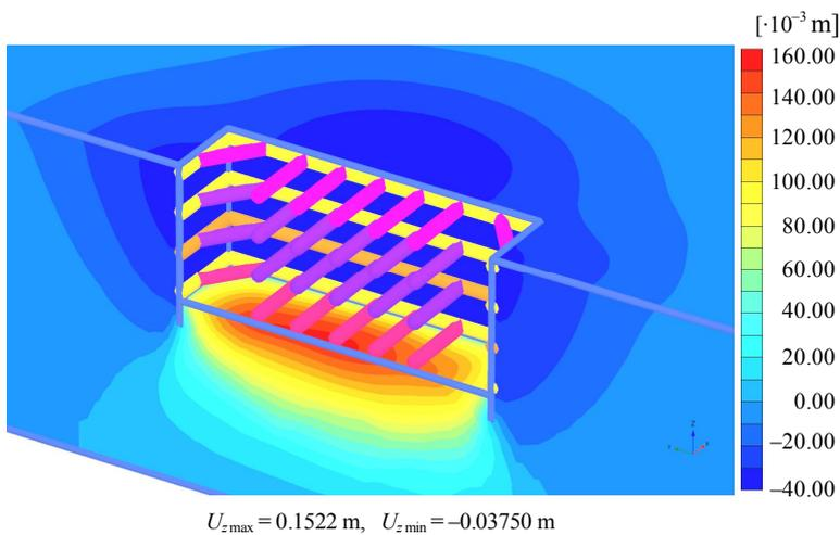
Fig.5. Surface shift troughs for excavation with 40 m length in sandy soil (Plaxis 3D)
