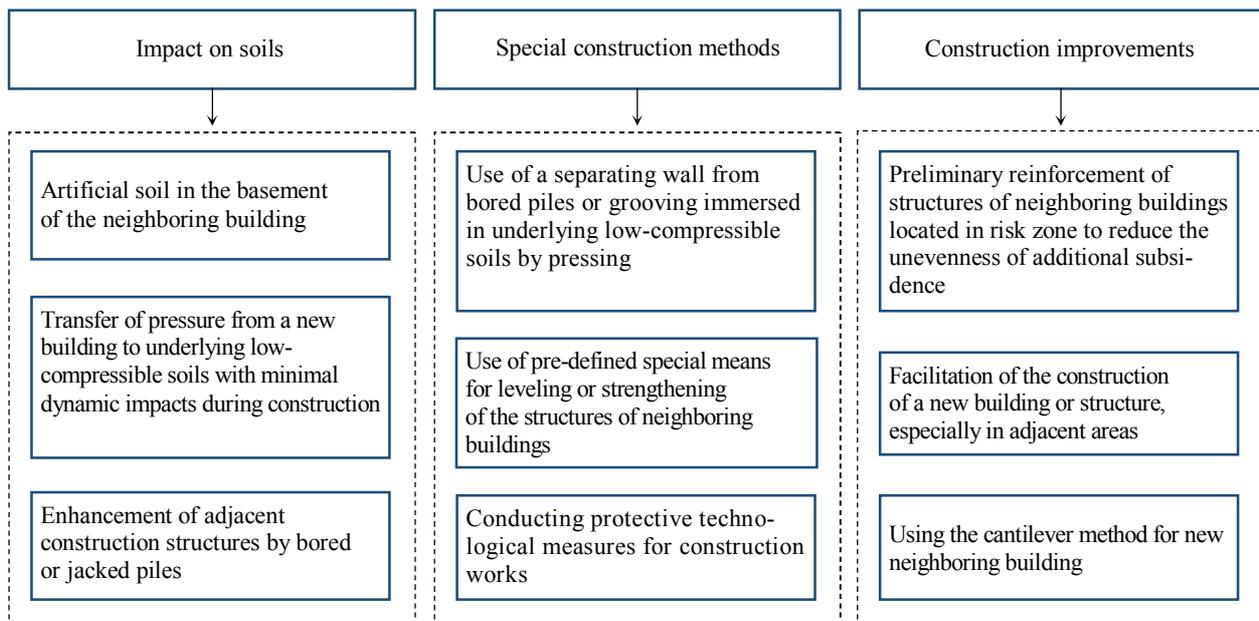
Fig.2. Classification of measures aimed at reducing the negative impacts from construction on neighboring buildings
