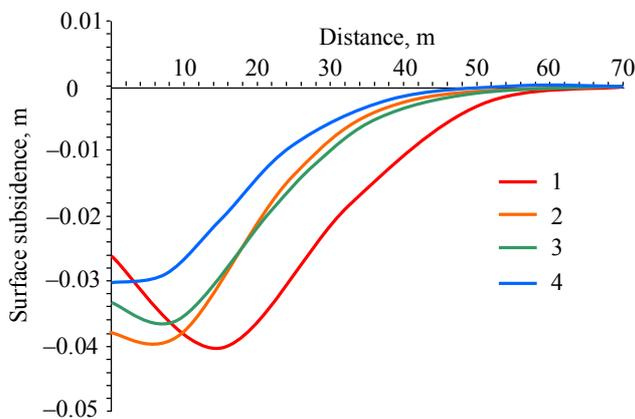
Fig.6. Graphs of vertical displacement of surface (depth of slurry trench is 800 mm) in clay N 1 for 2D (1) and 3D models with different excavation length (2-4 – 35; 30 and 40 m respectively)
