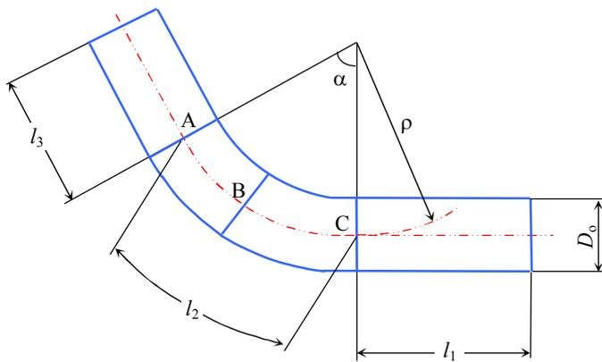
Fig. 1. The offset of the first type according to GOST 24950-81
