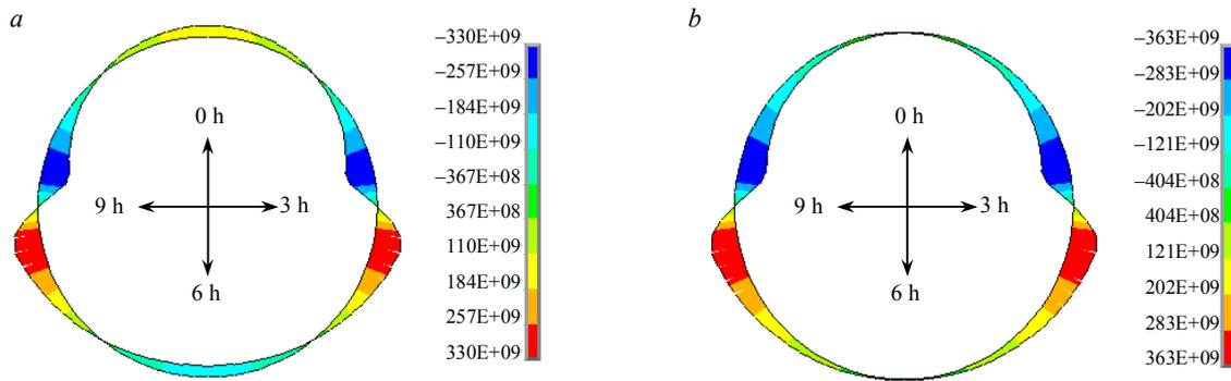
Fig.2. Distribution of longitudinal stresses in the middle cross-section of CBO
