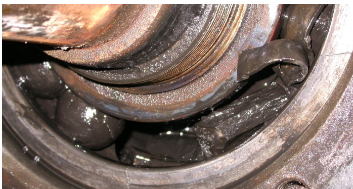
Fig.3. Destruction of the separator bearing pulp pump model GRaT 1800-67
