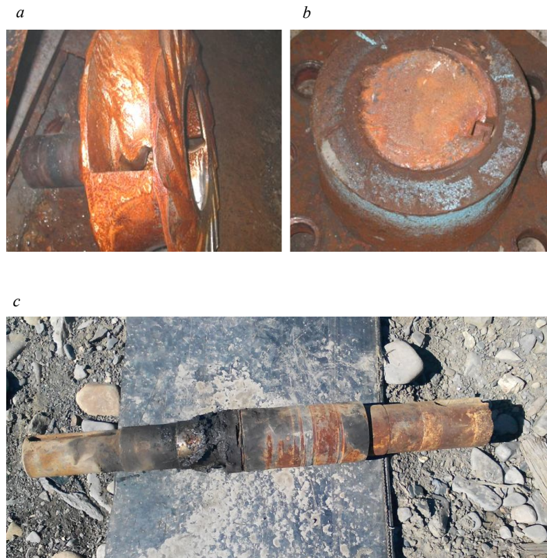
Fig.5. Kinks of shafts of centrifugal single-stage pumps: a, b – pulp pumps; c – «D»-type pump
