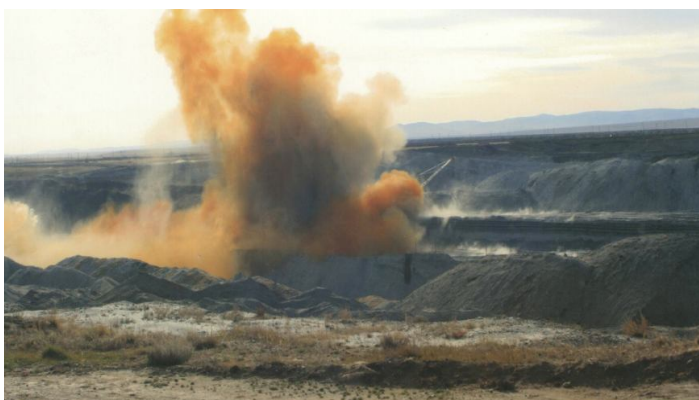
Fig.5. A photo of ANFO mixture (layered pie type) blasting charged by mixing-charging machine at Baganuur deposit
