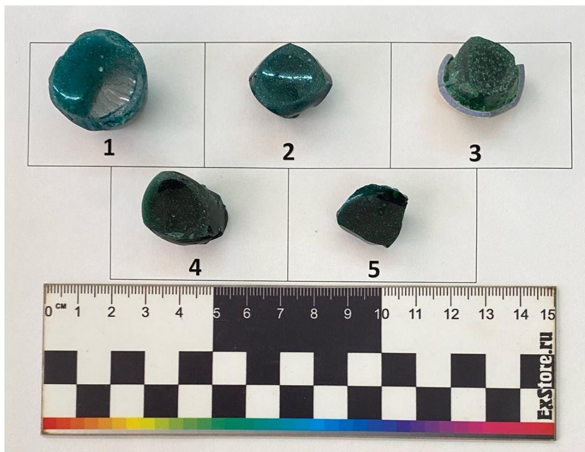
Figure 2. Calibration samples of enamel
