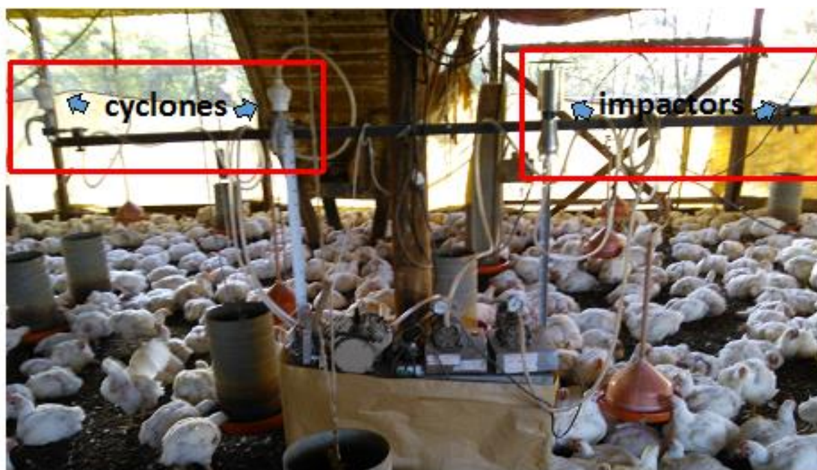
Figure 1. URG Cyclones, ZUF Impactor and Sioutas Personal Impactor collecting particulate matter in the commercial poultry house.
