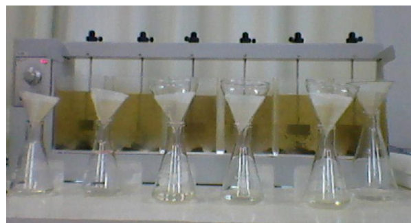
Figure 1. Jar test equipment and filtration system of the effluent after coagulation.
