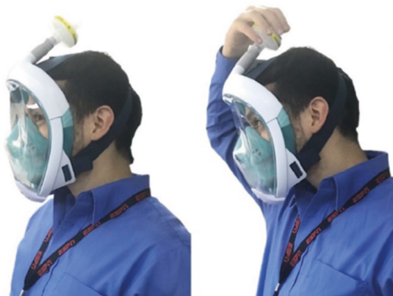
Figure 1. Manual seal test on inspiration and exhalation
