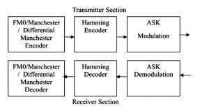
Fig. 1 - DSRC transceiver System
