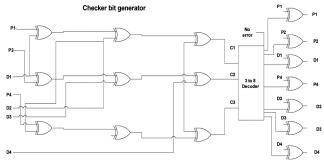
Fig. 3 — Hamming decoder circuit
