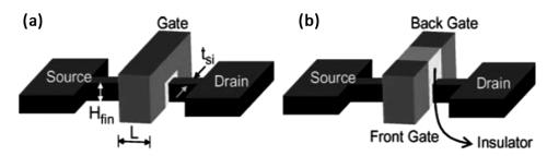
Fig. 7 — FinFET structure (a) shorted gate and (b) independent gate
