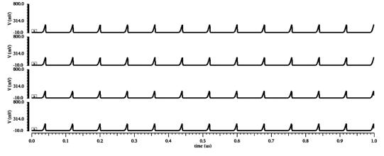
Fig. 8 — Simulation results of parity bit generator P1P2P4P8 (0000)
