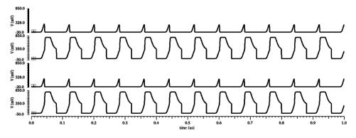
Fig. 9 — Simulation results of checker bit generator C8C4C2C1 (1010)
