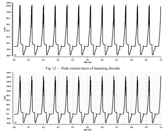
Fig. 13 — Peak current traces of hamming CODEC
