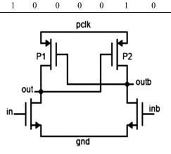
Fig. 4 — ECRL buffer/ inverter
