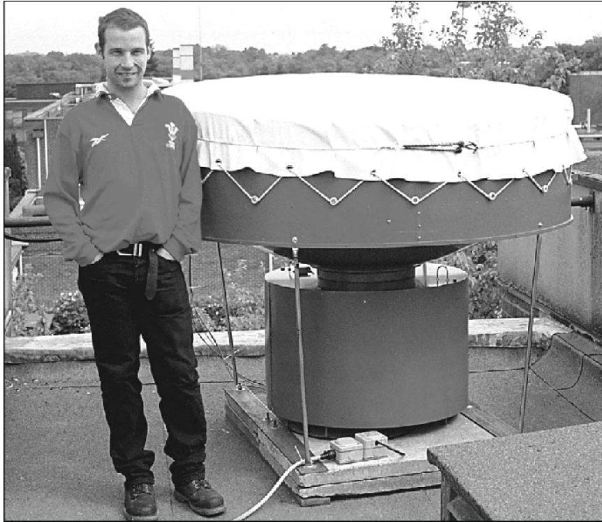
Figure 1.7 Shown beside Professor Jason Chapman is the entomological vertical-looking radar (VLR) device on the roof of the Plant and Invertebrate Ecology Division building at Rothamsted.
