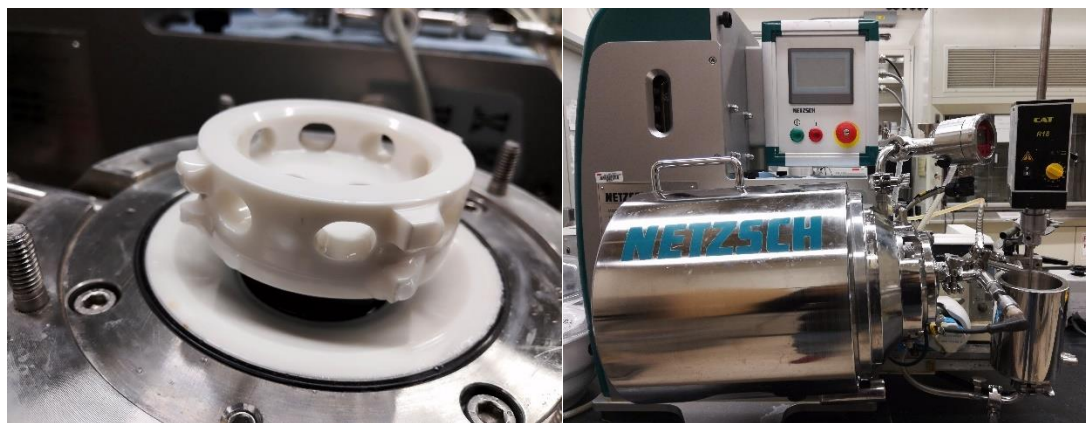
Figure 1.2 A ceramic (YSZ) stirrer with mixing elements at the periphery (left) inside a Netzsch Microcer horizontal wet stirred media mill used in the experimental work (right).
