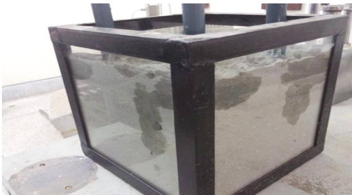
Figure 8: Permeation of grout occur
