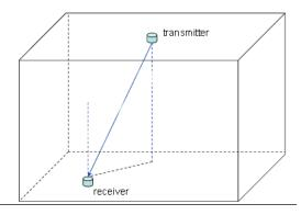
Figure 1: Geometrical Representation of non-directed LOS of VLC
