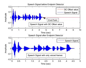
Fig. 3. Graphical representation of Endpoint detection process
