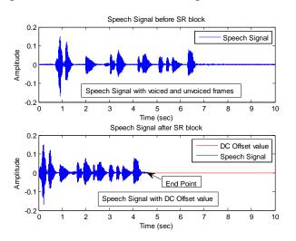
Fig. 2. Graphical representation of silence removal process
