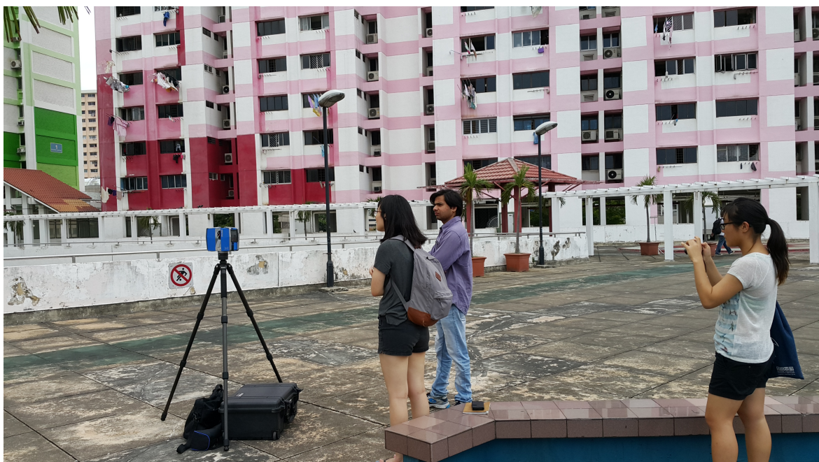
Image 3. 3d point cloud scanning of the Rochor Centre in Singapore. Image Credits: Felix Raspall
