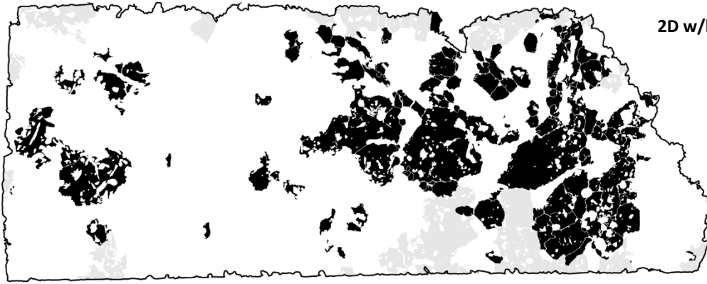
Figure C.39 – Binarised image used to calculate hornblende CSDs in sample M4 B. Grey crystals indicate those truncated by the boundary of the thin section and thus excluded from analysis. Inset histogram visualises the aspect ratio distribution of the measured population (black line), against that of the best fitting shape estimate (grey area).
