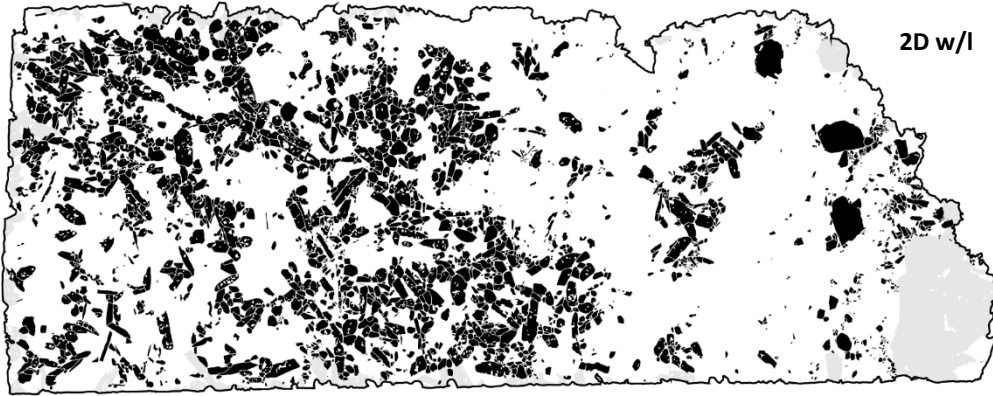
Figure C.37 – Binarised image used to calculate clinopyroxene CSDs in sample M4 B. Grey crystals indicate those truncated by the boundary of the thin section and thus excluded from analysis. Inset histogram visualises the aspect ratio distribution of the measured population (black line), against that of the best fitting shape estimate (grey area).
