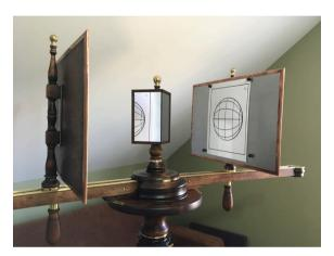
Fig. 16 Wheatstone Stereoscope. This is my second attempt at a stereoscope. It is in homage to Wheatstone's devices rather than a replica. The pivoting arms and circular forms are inspired by the idea of an orrery.
