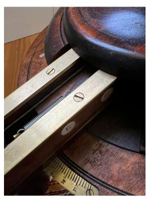
Fig. 15 Rigging Channel. The two image-plates are connected through the centre of the stereoscope by wires. When you pull or push one image-plate the other is pushed or pulled symmetrically. Note the "ivory" inlay on the side of the arm (made from deer antler rather than elephant tusk).
