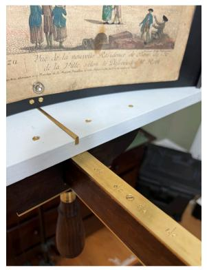
Fig. 10 Optical Theatre: Moveable Image Plate. Here you can see the track along which the image-plate can move and the adjusting handle below. You can also see how the image-plate can be curved or, by adjusting the knob at the back, be allowed to flatten again.
