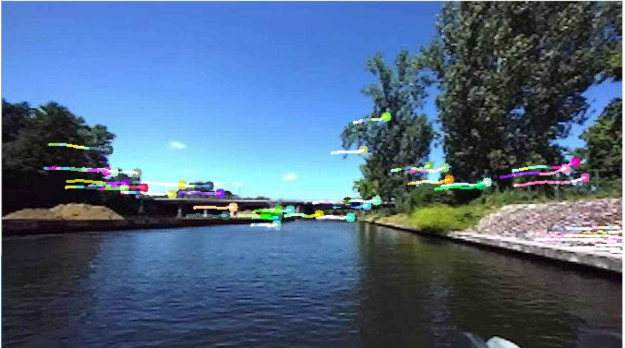
Figure 4.7: The Lucas-Kanade algorithm is implemented on the RGB images gained during the measurement campaign. The dots and lines indicate significant geometrical features recognized and tracked by the algorithm.
