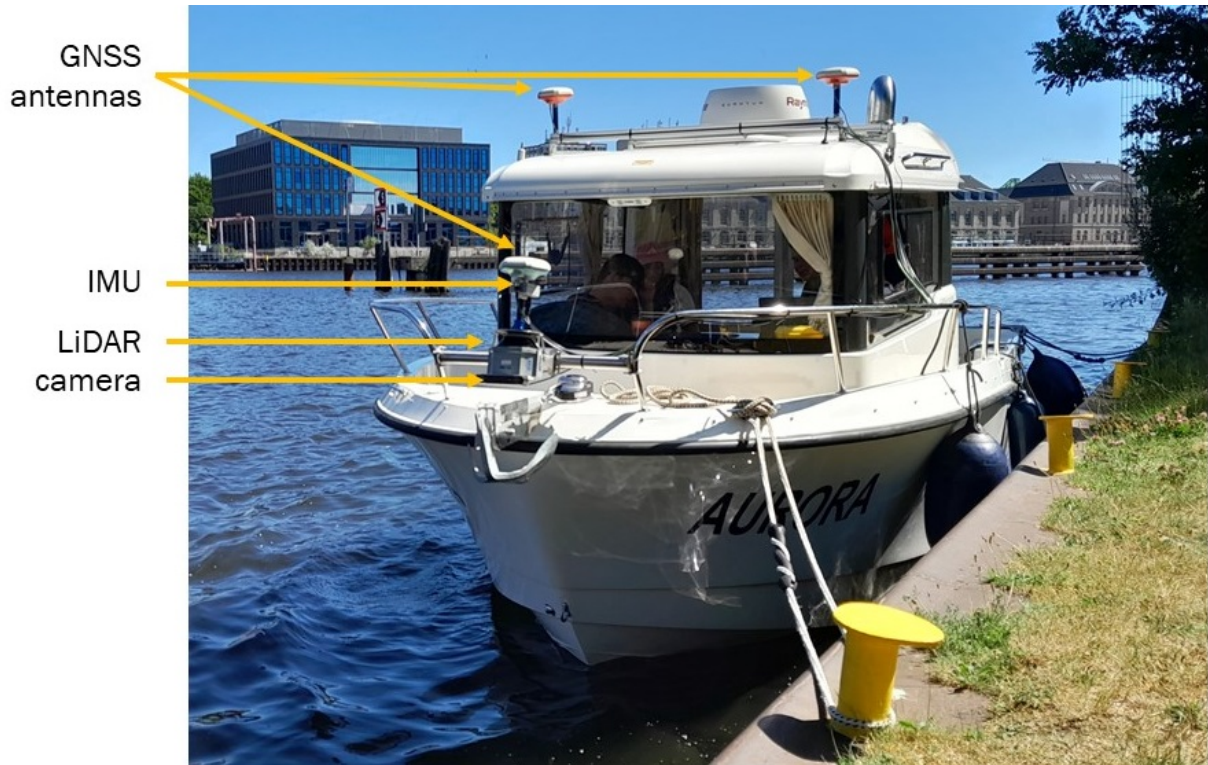
Figure 3.4: The motorboat Aurora was used for the measurement campaign. The optical sensors, IMU and one GNSS antenna were mounted on the bow of the boat and two further GNSS antennas on the roof.
