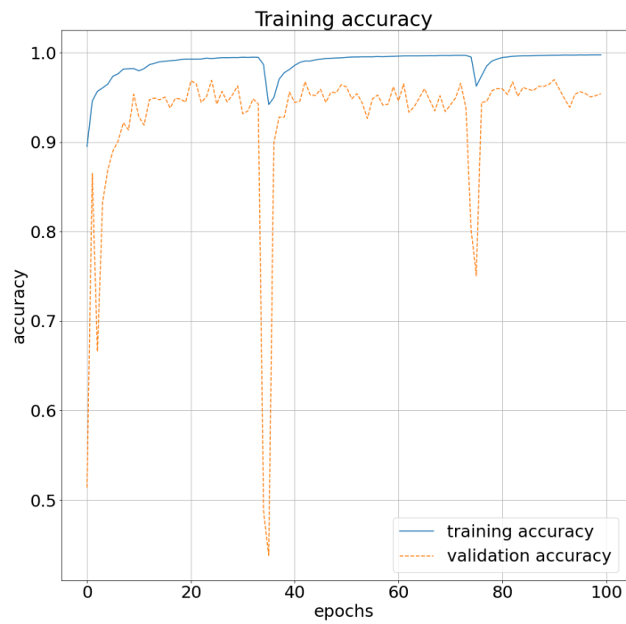
(a) Accuracy over 100 epochs. The introduced spikes might be the effect of the small dataset.
