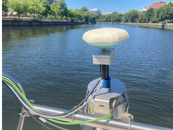
Figure 3.5: The sensor combination at the bow of the boat consists of a GNSS antenna, an IMU, the LiDAR sensor and a stereo camera (top-down).
