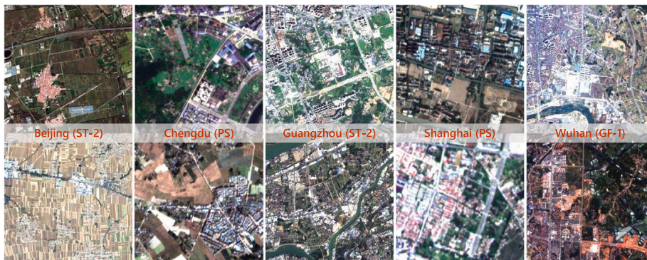
Fig. 4. Each column indicates images from the same city. There are obvious spectral shifts even between images within the same city due to differences in imaging illumination and season. In addition, spatial resolutions of different data sources are distinctly diverse. These heterogeneities pose huge challenges to land cover mapping.
